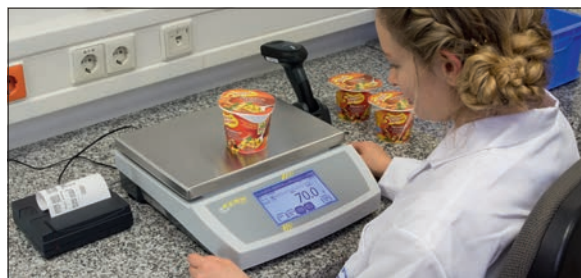
Sample testing of a pre-packaged item with an average tare value, e.g. the relative constant packaging weight is entered as a fixed value
