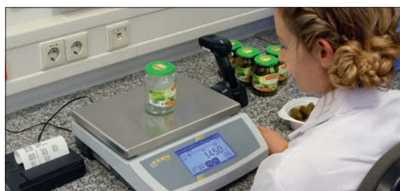
Sample testing of a pre-packaged item with fluctuating packaging weight, such as glass containers, e.g. the tare weight is entered individually for each sample.
