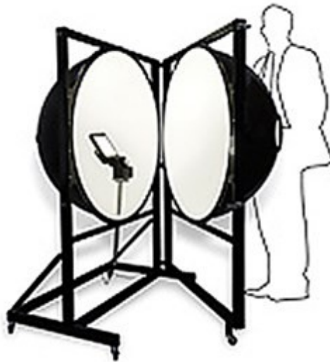
Gossen M601E Mavosphere 1100 Integrating Sphere ID 1100mm
