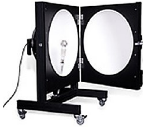
Gossen M601D Mavosphere 500 Integrating Sphere ID 500mm
